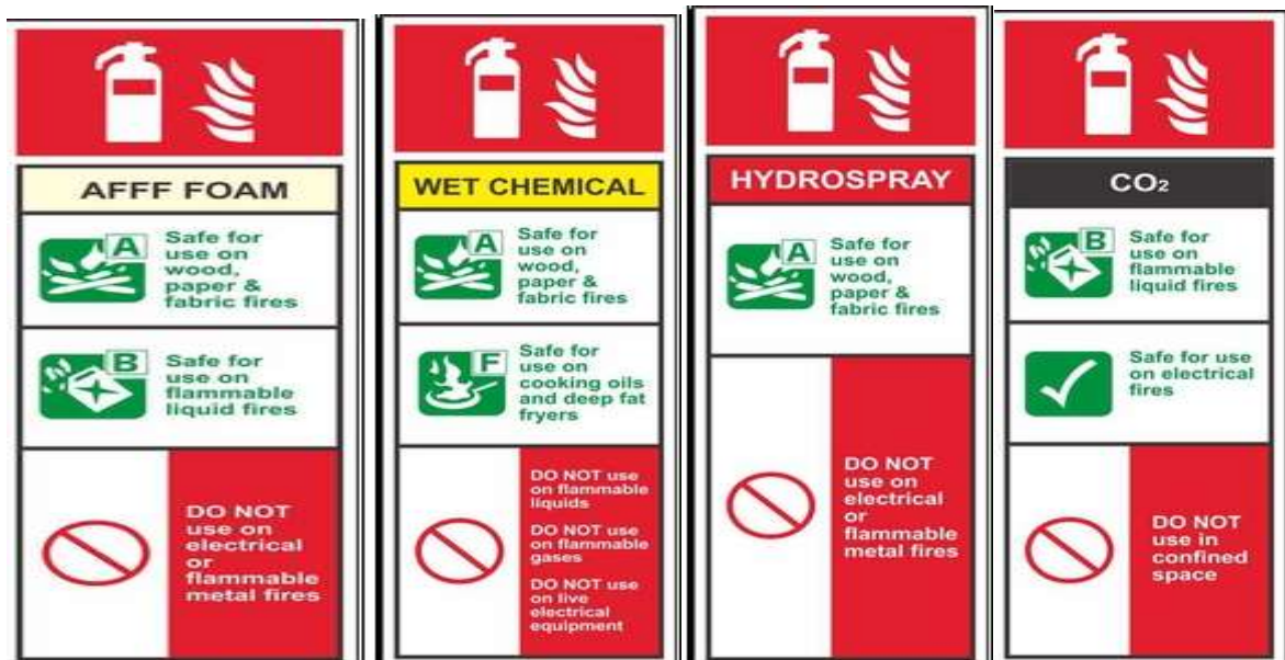
Figure 60: Signs for different types of fire extinguishers.
