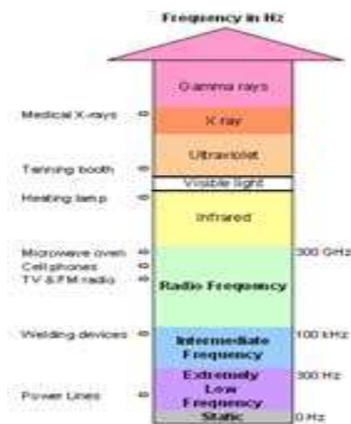
Figure 54: Frequency ranges of electromagnetic fields
