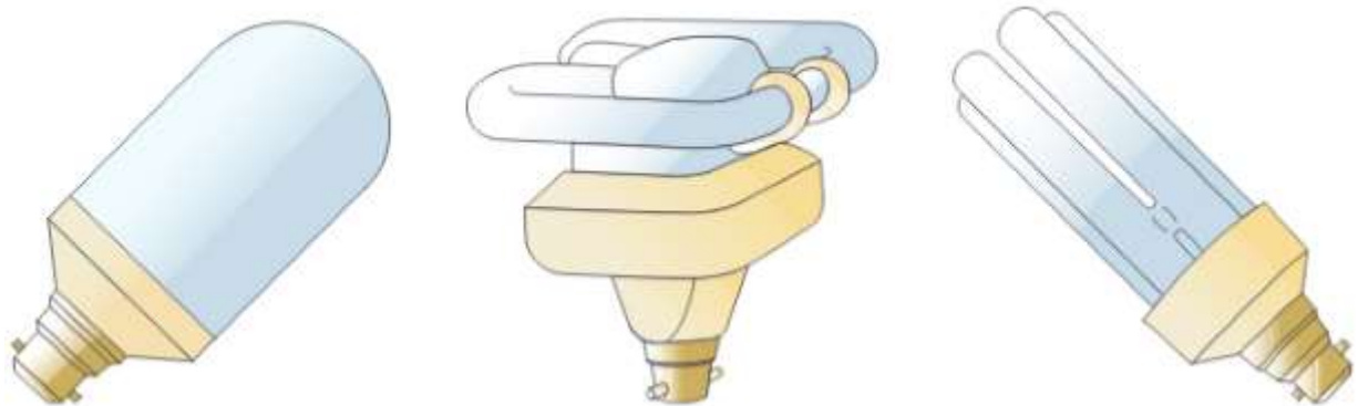
Figure 273 Energy efficient lamps
