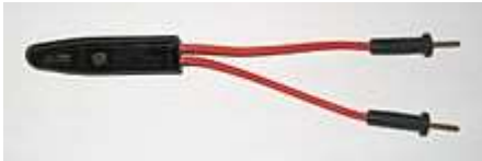
Figure 311 Neon test lamp for line voltage
