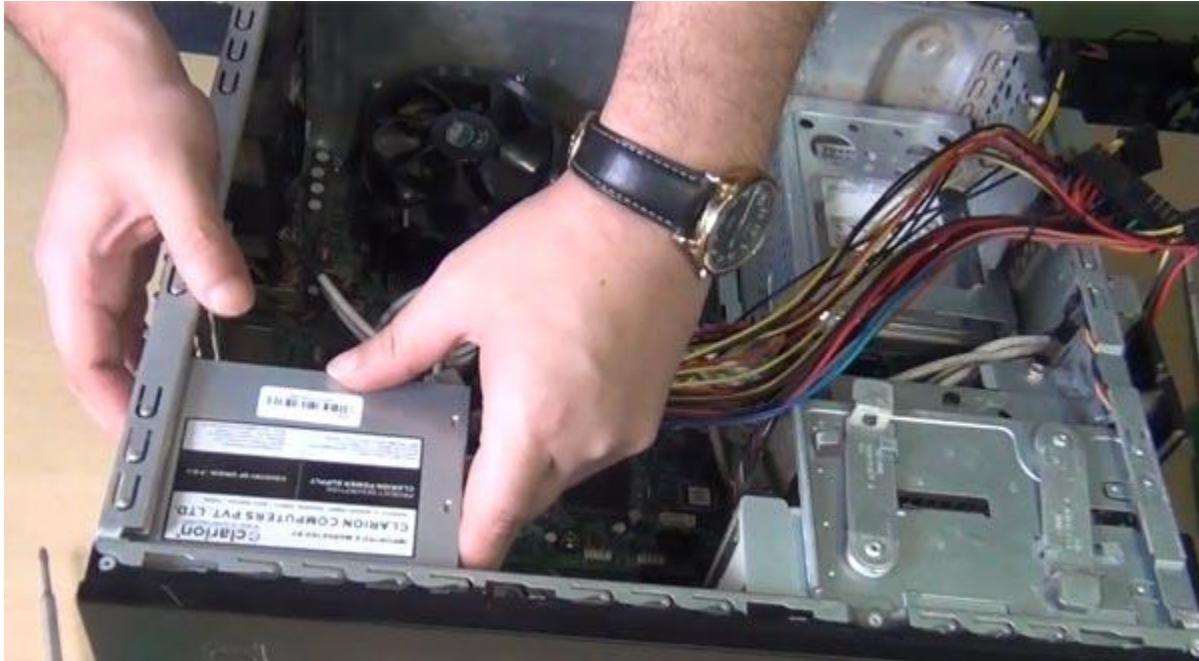
Figure 14 Installing SMPS (Power supply unit)
